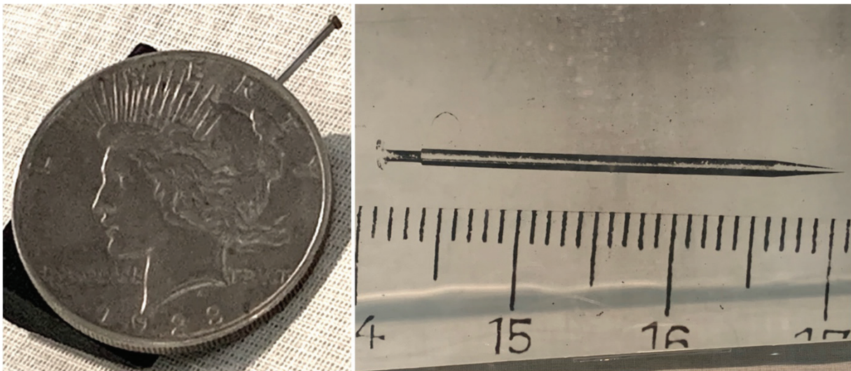
Left: Poison pin silver Peace dollar of the type given to Capt. Francis Gary Powers. Right: poison pin imbedded in the silver Peace dollar and coated with curare. Photographs by the author.
